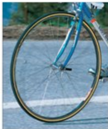
Above: Narrow-section racing wheel.
